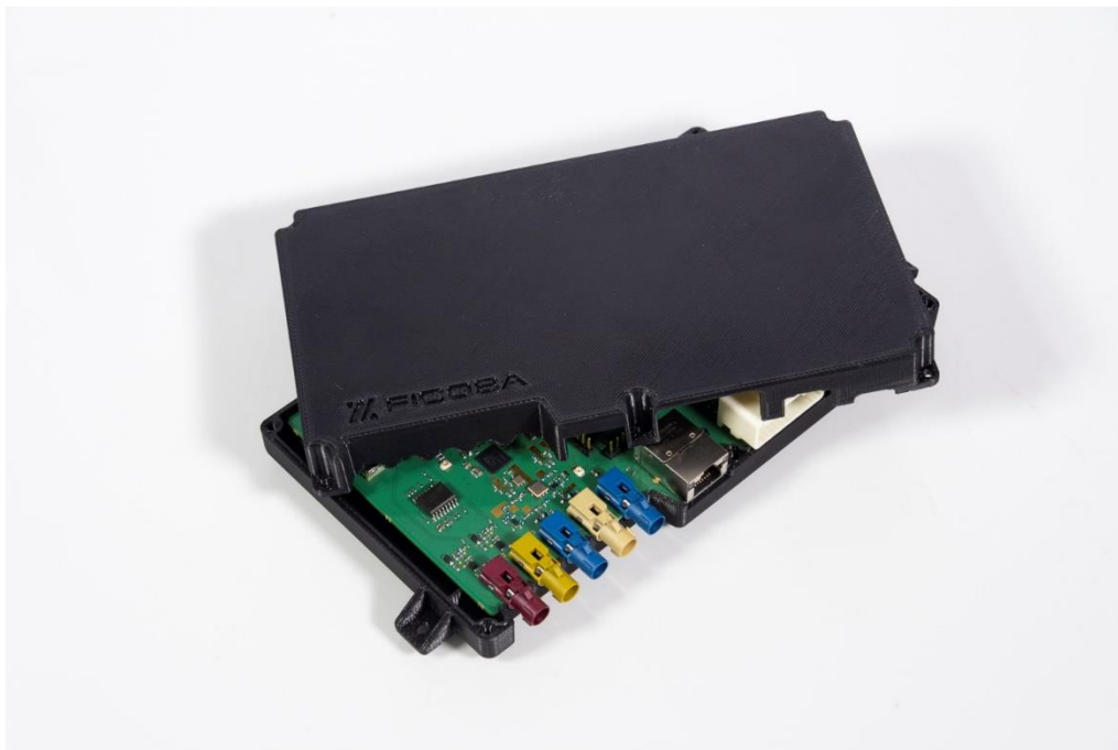
The ESCAPE GNSS Engine board in its final packaging (courtesy of FICOSA)
